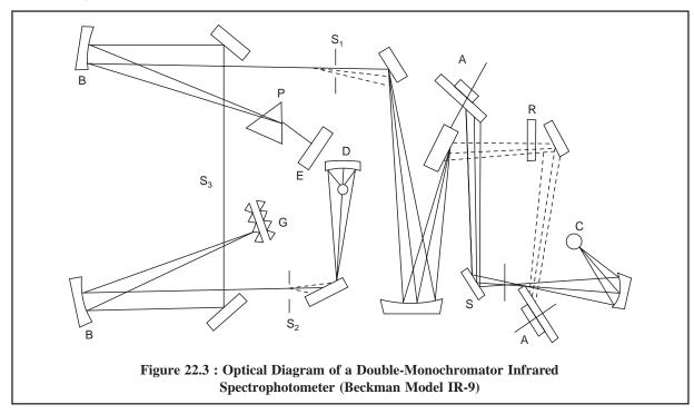
The various components of a double-monochromator infrared spectrophotometer shown in Figure 22.3 are as follows below :
