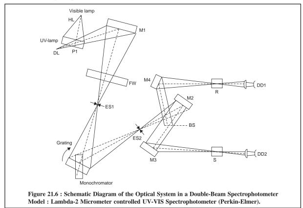
The various components of Figure 21.6 are stated below :
