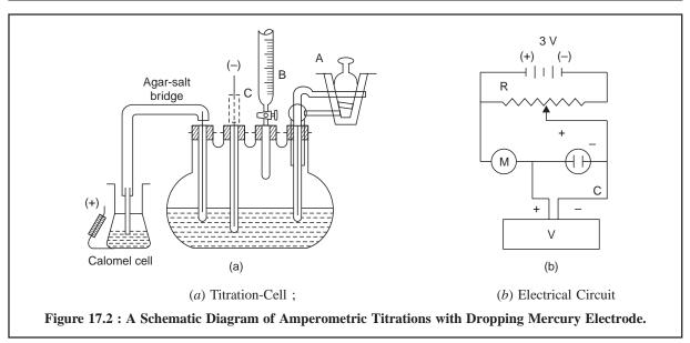
For Figure : 17.2 [a]For Figure : 17.2 [b]A = 2-Way gas-inlet tube, $R = Potential divider (a 50 - 100\Omega variable resistance),$ B = Semimicro burette (graduated in 0.01 ml), and<math>C = Cell, $M = Micro-ammeter (\mu A), and$  $M = Micro-ammeter (\mu A), and$ C = Dropping mercury electrode.<math>V = Digital voltmeter.The following steps may be carried out in a sequential manner for an amperometric titration,
