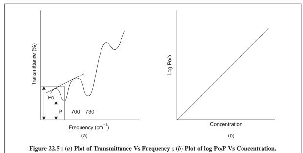
The value of the incident radiant energy Po may be achieved by drawing a straight line tangent to the spectral absorption curve at the position of the analyte's absorption band. Consequently the transmittance P is usually measured at the point of maximum absorption. Finally, the value of log Po/P is plotted against the concentration as shown in Figure 22.5.
