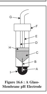
solution having a fixed composition *e.g.*, aqueous  $CaCl_2$  saturated with AgCl (C). The liquid calcium di (*n*-decyl) phosphate,  $[{CH_3(CH_2)_8CH_2O}_2PO_2]_2$  Ca serves as the membrane, positioned at the lower end of the electrode, and strategically immobilized by a thin disk of PVC (polyvinyl chloride) (A) which is not penetrable with water.
