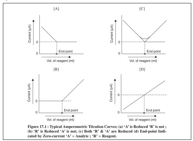
**Figure 17.1 (b) :** It designates typical of an amperometric titration curve wherein the reagent exclusively reacts at the microelectrode surface and the analyte does not. In other words, the reagent gives rise to a diffusion current, whereas the solute does not ; it means an electro-active precipitating reagent is being added to an inactive substance.
