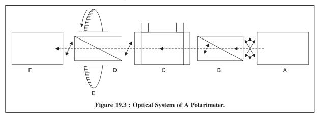
Figure 19.3, represents the optical system of a polarimeter,
