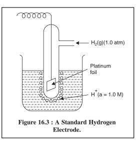
usual convention to assign the potential of SHE a value exactly equal to zero at all temperatures.
