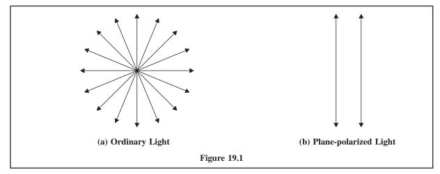
A few crystalline substances, for instance : Iceland spar, Calcite (a form of CaCO<sub>3</sub>) or Polaroid, possess different refractive indices for light whose field oscillates either perpendicular or parallel to the principal plane of the crystal. Thus, an ordinary light (unpolarized light) gets converted into a plane-polarized light by simply passing it through a lens made of the above cited materials and traditionally called a **Nicol prism** (after **William Nicol-the inventor**).
