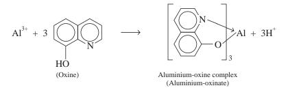
The resulting precipitate of aluminium-oxine complex is crystalline in nature and hence can be filtered conveniently, washed with water and finally dried at 130-150°C to constant weight.
